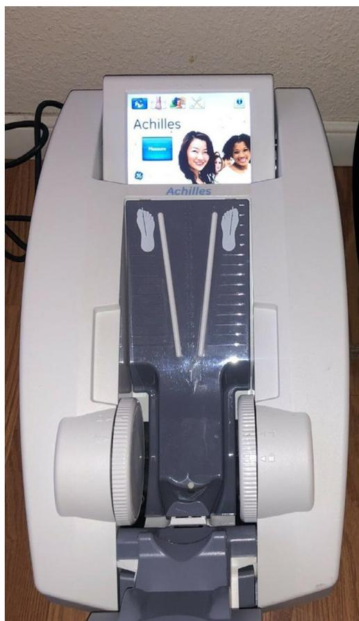
Fig. 5. Achilles Express II bone ultrasonometer.
